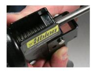
**STEP 3:** Push rod thru the spring and out the other rod hole. It may be necessary to locate the spring by inserting a screwdriver thru the front rod hole.
