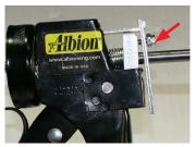
**STEP 6:** Make final adjustments to the adjustment screw for smooth operation. Note that the hinge pin can be located for high or low thrust applications.
