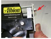
**STEP 5:** Insert link into handle and attached thumb release. Press-in thumb release so rod and grip plate can be positioned in-line with each other. If the rod will not retract, try tightening the adjustment screw and/ or turn the rod while pushing it thru. If the problem continues, there may be a burr on the rod, preventing installation. Check to make sure rod will fit over grip plate.
