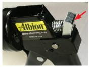
**STEP 4:** Place the steel bushing onto rod so it contacts the inside grip plate. Push the rod forward even with the bushing (as shown). Insert the spring over the bushing and install rear grip plate. Note the chamfer location on the grip plate. Press-in the upper area of the grip plate so the rod can retract enough to hold the grip plate in place.
