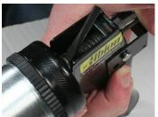
**STEP 2:** Make sure the trigger is completely forward (the main spring includes two springs nested together). Position the rod so that the spring ID will rest over it. Place a screwdriver into the 2nd winding of the spring (as shown) and push down, while collapsing the spring into place.
