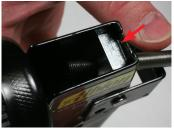
**STEP 1:** Insert rod thru handle hole and place grip plate onto rod. Note that the gripping plate chamfer is to be located towards the rear of the handle. (See arrows)
