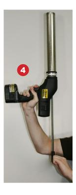
IMPORTANT: Do not take barrel off without taking piston packing apart first. Assemble packing while barrel is attached to handle.
