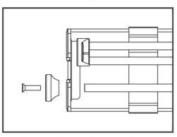
Step 1. Remove large ejector from left side
