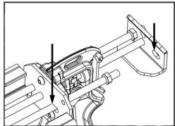
Step 3. Move rod to inner position on back plate and pull. Re-tighten rod and crown nut to pull on the inner position.
