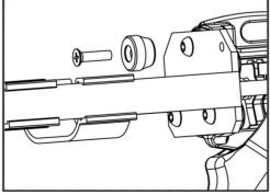
Step 4. Remove small ejector from backplate and replace with large ejector. Use the long screw to attach ejector to backplate.
