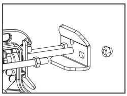
Step 2. Remove crown nut and rod from pull
