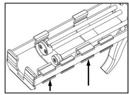
Step 5. Attach small ejector to rod. Place 75ml cartridge snaps inside the carriage as shown.
