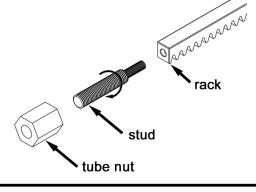
Step 2. Screw tube nut onto stud until it seats onto the rack.
