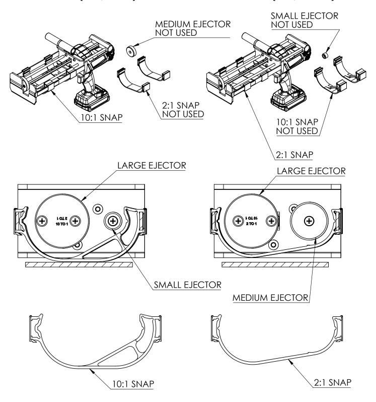
LARGE EJECTOR IS USED FOR BOTH SET-UPS. FLIP EJECTOR TO CORRECT POSITION FOR USE WITH EITHER 750/75ML OR 600/300ML CARTRIDGES. EJECTORS SHOULD BE CONCENTRIC WITH INSIDE OF STRAP WHEN PROPERLY INSTALLED.
