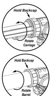
If rod is stuck and will not disengage automatically, press and quickly release the trigger. Then, press the control switch and slowly pull back on the rod.
