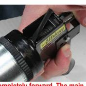
Step 2: Make sure the trigger is completely forward. The main spring includes two springs nested together. Position the rod so that the spring I.D. will rest over it. Place a screwdriver into the 2nd winding of the spring (as shown) and push down, while collapsing the spring into place.
