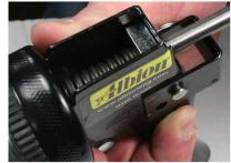
Step 3: Push rod thru spring and out other hole. It may be necessary to locate spring by inserting a screwdriver thru the front rod hole.
