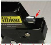
Step 4: Insert steel bushing onto rod so it contacts the inside grip plate. Push the rod forward even with the bushing (as shown). Insert spring over bushing and install rear grip plate. Note the chamfer location on the grip plate. Press-in the upper area of the grip plate so the rod can retract enough to hold the grip plate in place.
