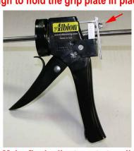
Step 6: Make final adjustments to adjustment screw for smooth operation. Note that the hinge pin can be located for high or low thrust applications.
