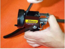
Step 6 Slide spring into position. Make sure spring is centered about the handle hole, then push rod forward. Remove screw driver and push rod thru handle hole.
