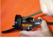
Step 5 While compressing spring with screwdriver, push downward.
