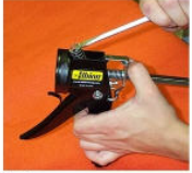
Step 4 Place spring onto rod, make sure trigger is forward. Place screwdriver behind first coil of spring.
