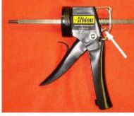
Step 7 The handle is assembled. The adjustment screw can be adjusted if there is too much play in the trigger or if the rod is difficult to pull back.
