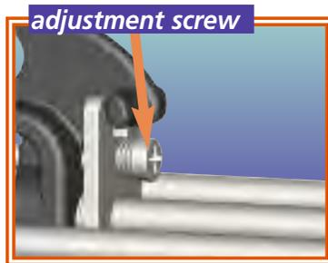
life of the gun—as the tool wears you can adjust the screw to eliminate wasted motion.
