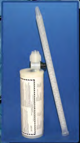
CoAxial Cartridge 7-1/2" x 2-1/2" 380ml 10:1 mix ratio
